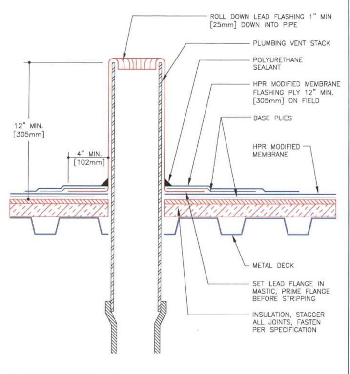
ALL PLIES SET IN BITUMEN SEE SPECIFICATIONS FOR SURFACING
