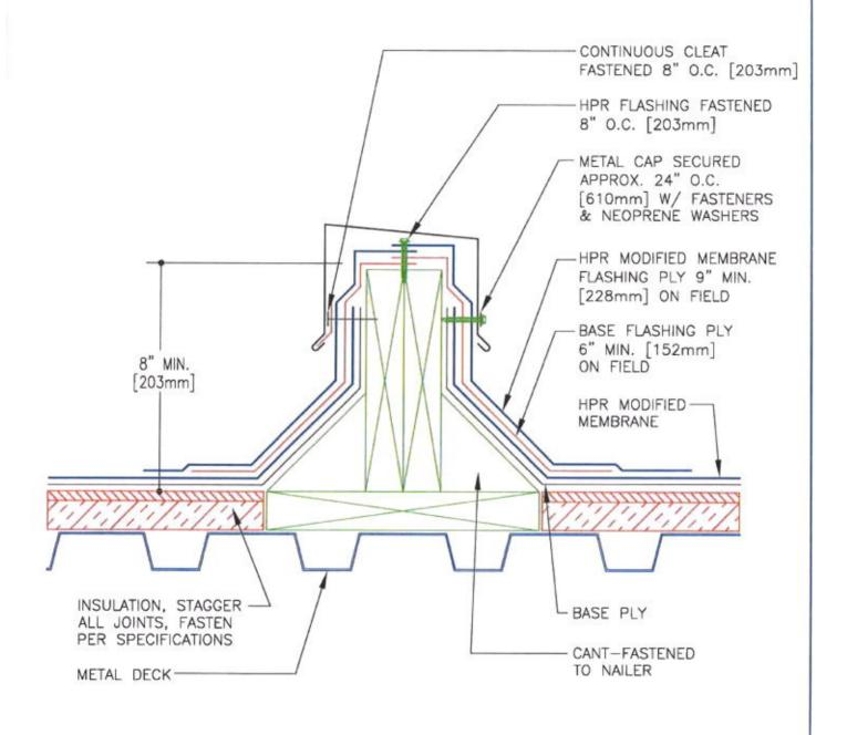
ALL PLIES SET IN BITUMEN SEE SPECIFICATIONS FOR SURFACING
