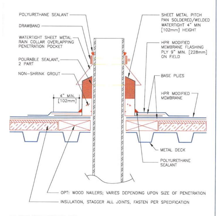
ALL PLIES SET IN BITUMEN SEE SPECIFICATIONS FOR SURFACING
