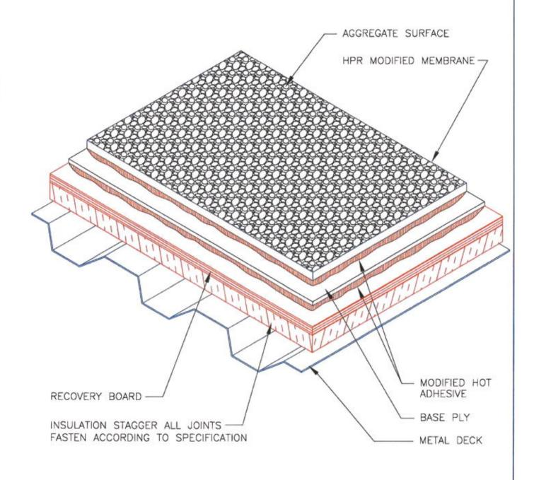
ALL PLIES SET IN BITUMEN SEE SPECIFICATIONS FOR SURFACING
