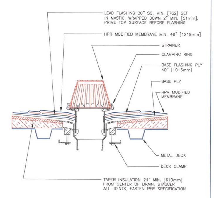
ALL PLIES SET IN BITUMEN SEE SPECIFICATIONS FOR SURFACING
